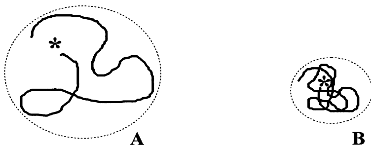
Fig. 1. Two macroradical coils having the same kinetic chain length with expanded (A) and shrunk (B) conformations. Thermodynamic and steric excluded volumes determine the process of the segmental diffusion in coils A and B, respectively.
